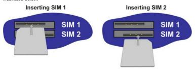
In both cases, the end of the SIM card with the chamfered corner should be inserted first. For SIM 1 the contacts should be face down. For SIM 2 the contacts should be face up.
